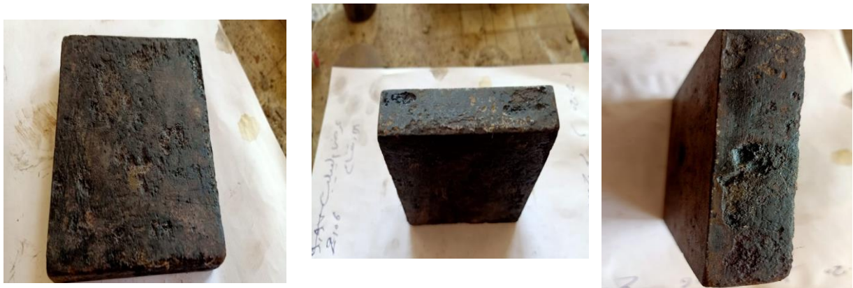
Figure 18: Effect of Salt Water in Experimental Model Steel Footing
