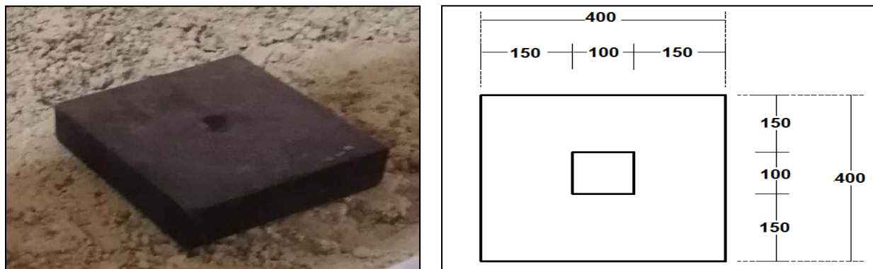
Figure 3: Steel Plate Footing
