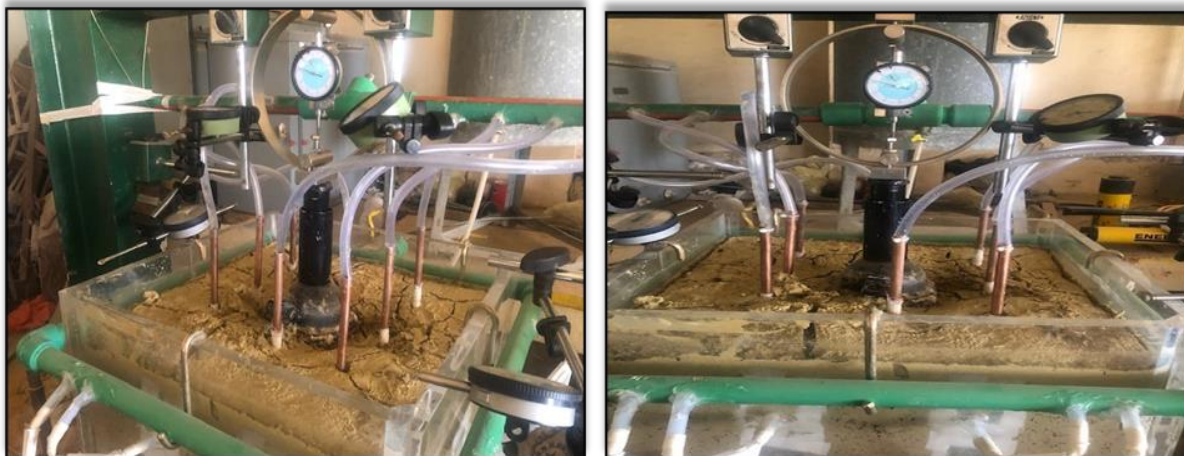
Figure 5: Salt Water Distribution System
