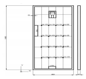
Fig. 3. The distribution of thermocouples on the PV cell's rear surface.
