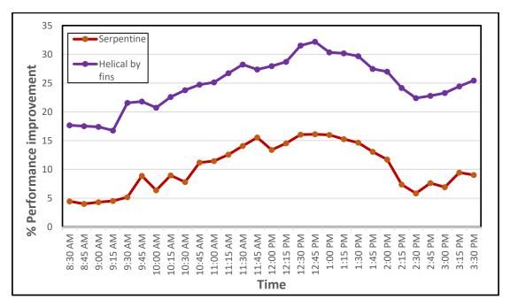
Fig. 8. Performance improvement in the electrical efficiency for serpentine shape and helical shape by fins at 2 LPM.
