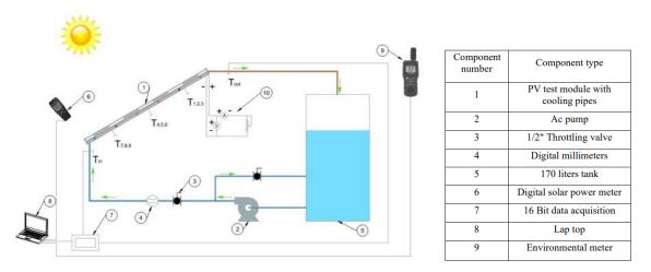
Fig.5. The PV cooling system in the experimental setup is depicted schematically.
