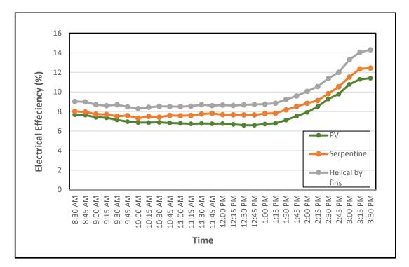
Fig. 7. During the daytime at 2 LPM, photovoltaic efficiencies of PV/T and PV modules were compared.
