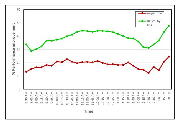
Fig. 14. Performance improvement in the electrical efficiency for serpentine shape and helical shape by fins at 6 LPM.
