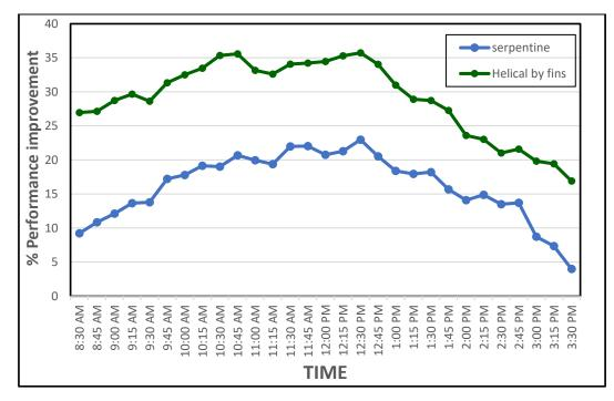
Fig. 11. Performance improvement in the electrical efficiency for serpentine shape and helical shape by fins at 4 LPM.
