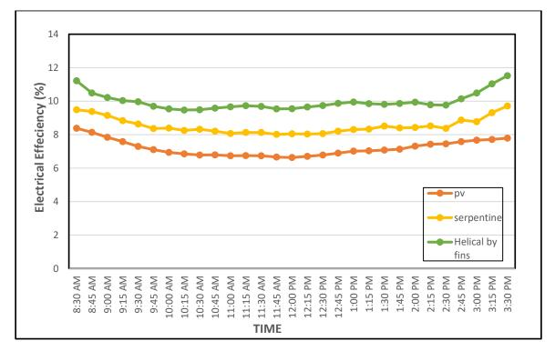
Fig. 13. During the day at 6 LPM, the photovoltaic efficiencies of the PV/T and PV modules were compared.
