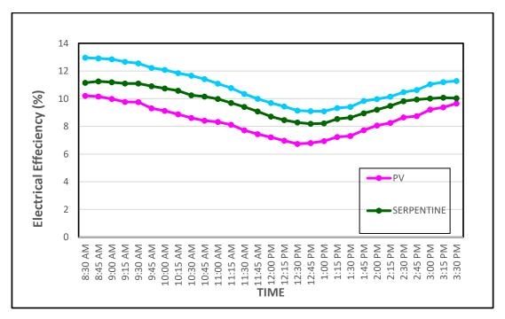
Fig. 10. During the day at 4 LPM, the photovoltaic efficiencies of the PV/T and PV modules were compared.
