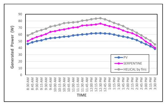
Fig. 9. PV module generated power, serpentine form and helical fins at 4 LPM.
