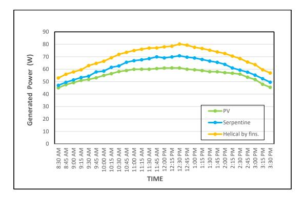
Fig. 6. At 2 LPM, generated power of PV module, serpentine form and helical by fins
