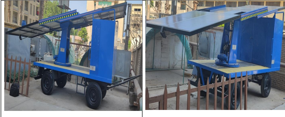
Fig. 3 Final View of the mobile solar water pumping system
