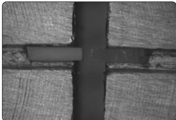
Fig. (5): Adhesive mode of failure for the micro-tensile bond strength inspected under the stereomicroscope.
