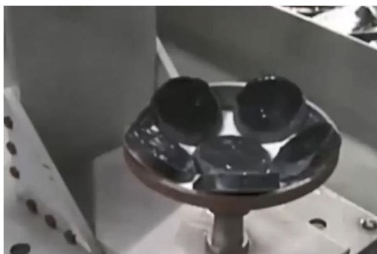
Figure 18. Lens after putting in the polishing machine.
