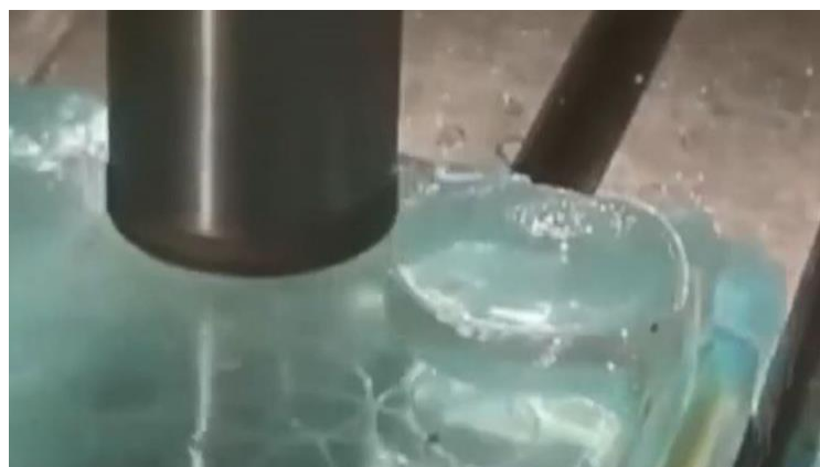
Figure 14. Real image of cutting from glass material to proposed lens array.
