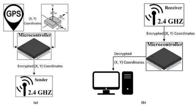
Figure 2. The transmission and the Receiver circuits. (a) The transmission Circuit (b) The Receiver Circuit.
