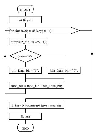
Figure 1. Flow Chart for CryptoBin Algorithm Structure.
