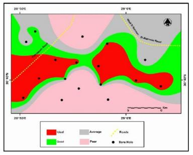
Fig. 9: Susceptibility of chloride ion distribution map (ppm) of the study area
