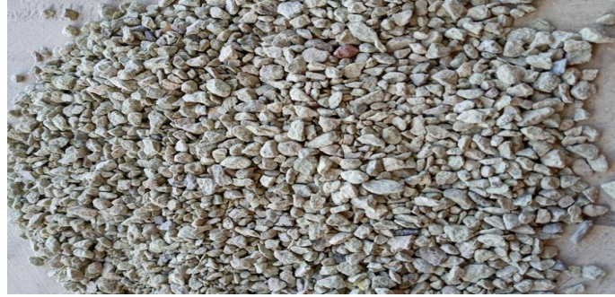
Figure 1: Commercial natural zeolite, clinoptilolite, granules (3-5mm)
