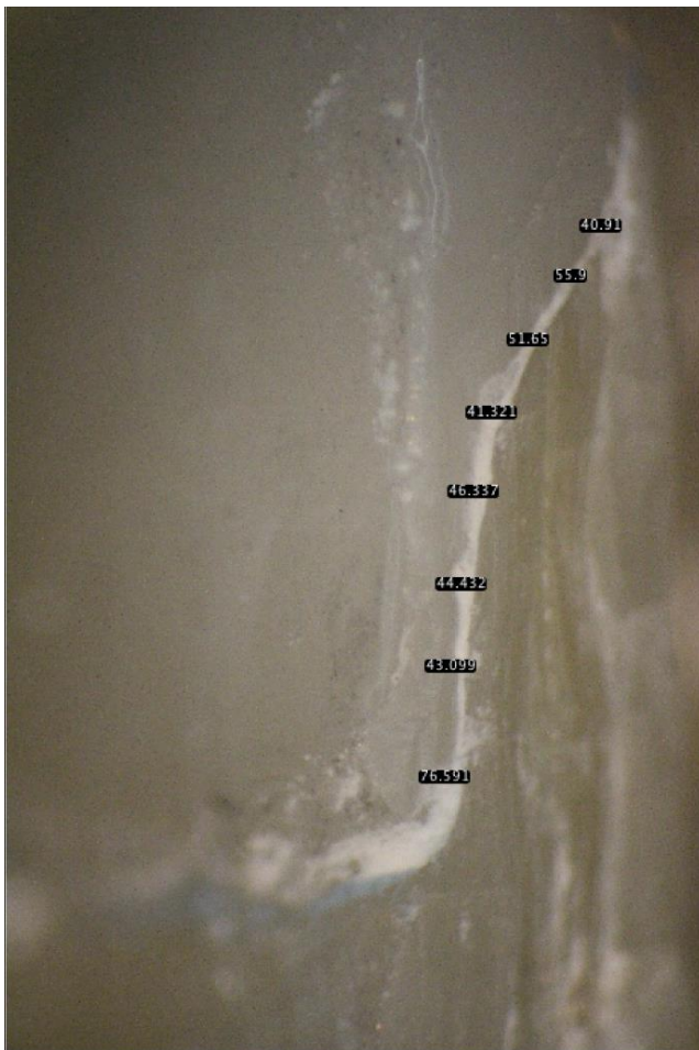
Figure 4. Measurement of the incisal external margin adaptation before thermocycling of e.max sample using image j software.
