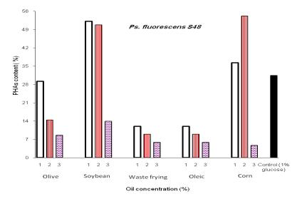
Fig. 4. PHAs production by *Ps. fluorescens* S48 as influenced by different concentrations of some vegetable oils and oleic acid after 72 hr of incubation at 30°C using shake flasks as a batch culture.
