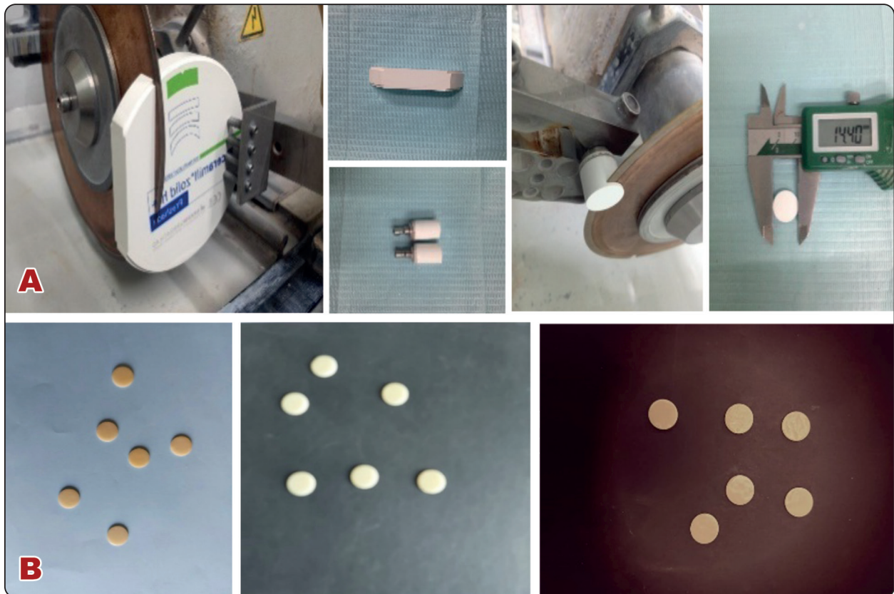
Fig. (1) a): Steps of construction of zirconia discs. b): The constructed discs
