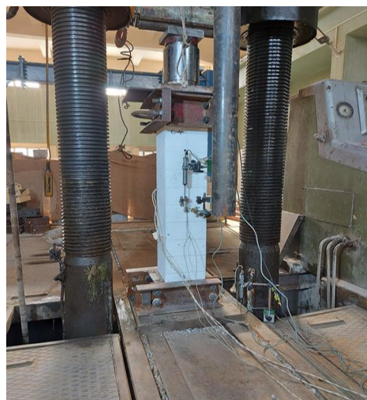
Fig. 8: Testing of column specimens
