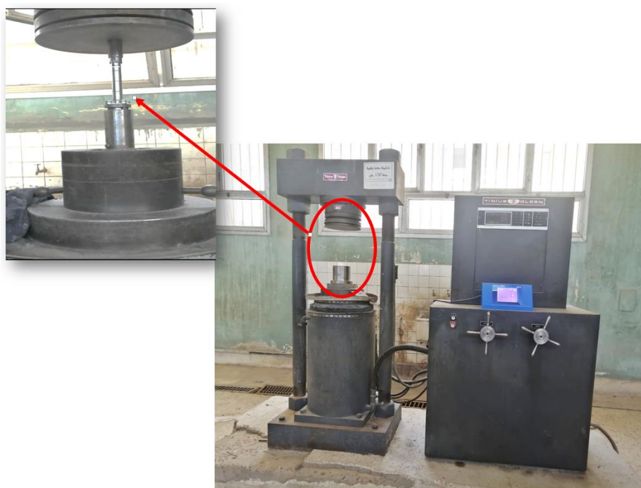
Fig. 2: Photo for experimental setup fixed on hydraulic press machine.
