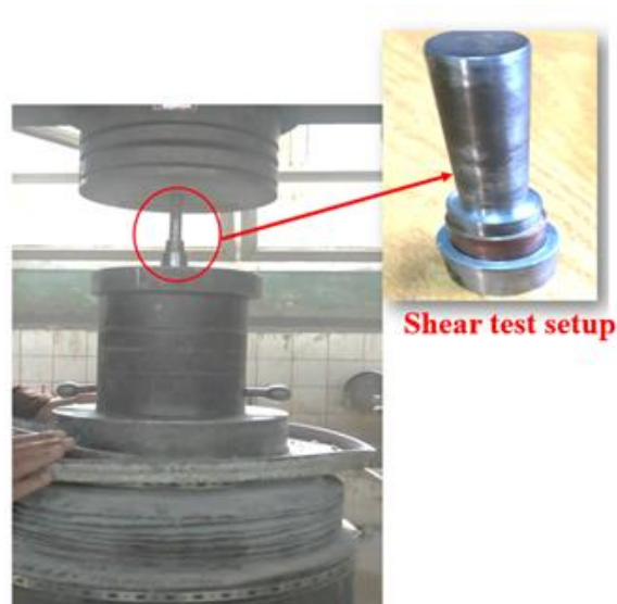
Fig. 4: Photo for experimental shear punch test setup fixed on hydraulic press machine.
