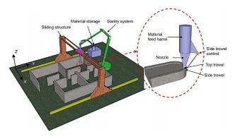
Fig. 5. Shows 3D printing during build construction MA GuoWei1, WANG Li & JU Yang" State-of-the-art of 3D printing technology of cementations material—An emerging technique for construction"2017-scince china- Technological Sciences
