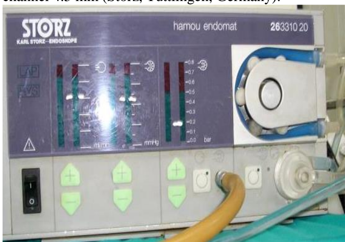
Figure (2): Continuous suction irrigation pump "Endomat".
