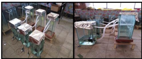
Photo (3): Experimental filtration set-up for metals Pb, and Cd removal by ceramic filters.
