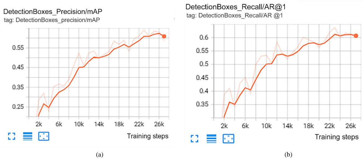
Fig. 100. Evaluation metrics for model B vs training steps: (a) Mean average precision (b) average recall on one detection per image.
