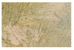
Fig.4Thin paint layer was applied on top of artificial cracks.
