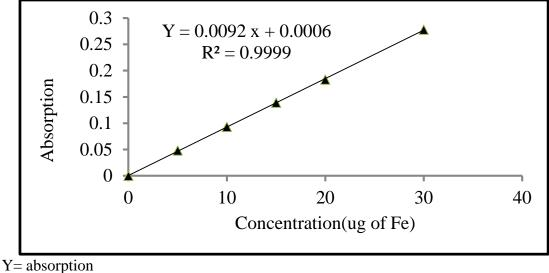
X = absorption X = concentration 0.0092 = slope of calibration graph0.0006 = Y- intercept
