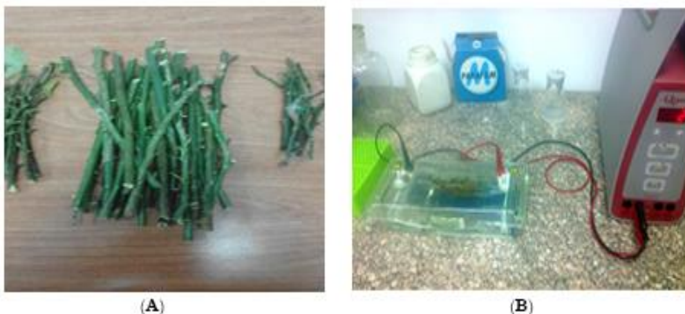
Fig. 3. Electrotherapy equipment used to produce virus-free plants in Citrus psorosis virus (CPsV). Stem segments with 3-5 buds used for therapy), single node explants prepared for grafting (A), Bio-Rad power supply and electrophoresis tank used for producing electric currents (B).
