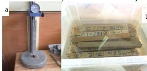
Fig. 3a Comparator used to measure the length of mortar bars Fig. 2b Specimen bars in sulphate solution for length change test
