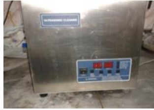
Fig.1 The used Ultra sonic Cleaner for dispersing nano particles in mixing water
