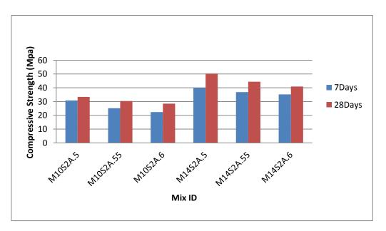
Figure 2: Effect of ratio of activator to fly ash
