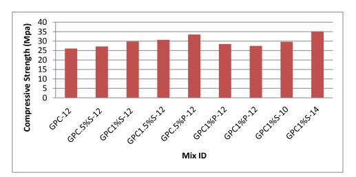
Figure 11: Compressive strength of GPC mixes at 28 days
