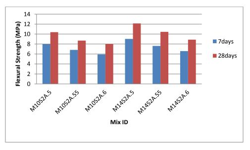
Figure7: Effect of ratio of activator to fly ash
