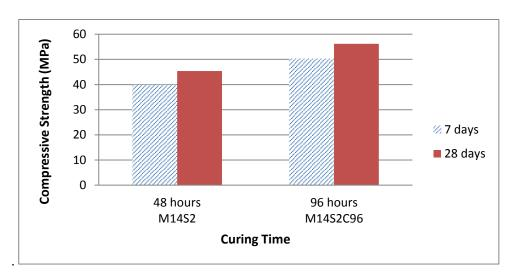
Figure 4 : Effect of varying the curing time
