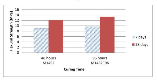
Figure 9 : Effect of varying the curing time
