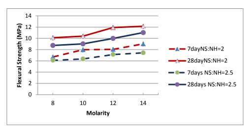
Figure 6: Effect of concentration of sodium hydroxide solution
