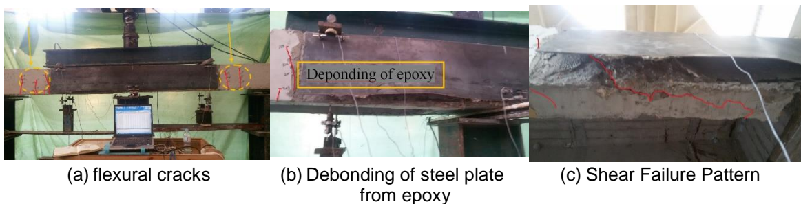
Fig. 13 Cracks mapping and failure pattern of beam B-ST.
