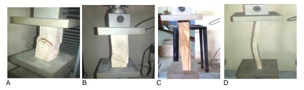
Figure 6: Typical shearing (A), crushing (B), splitting (C), and buckling (D) failure modes of timber samples oriented parallel to grain and under compression.
