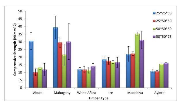
Figure 6: Compressive Strength for Varying Section of the Timber Samples
