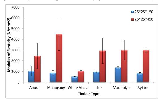
Figure 4: Elastic Modulus Results for Varying Sections of the Timber Species
