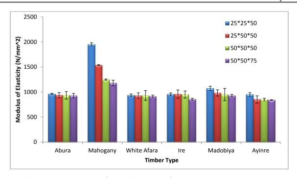
Figure 7: Elastic Modulus for Varying Section of the Timber Samples
