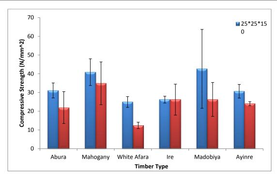
Figure 3: Compressive Strength Results for Varying Sections of the Timber Species
