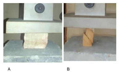
Figure 7: Typical crushing (A) and shearing (B) failure modes of timber samples under compression force perpendicular to grain.
