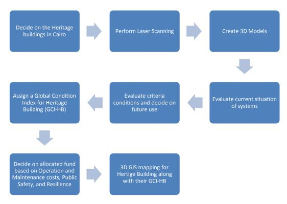
Fig. 1: Workflow of the Proposed HBIM framework
