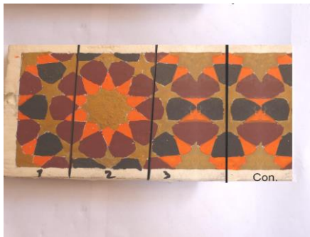
Fig. 11. Wood samples divided into four parts and sprayed with a mixed spore suspension (18 fungal strains) .
