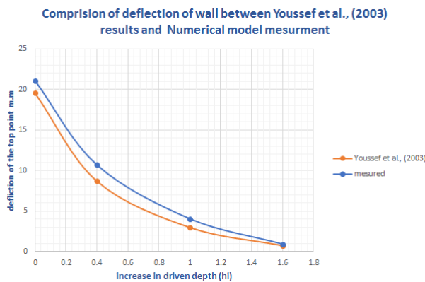
Fig. (3): Deflection of the Wall versus Increase of Driven Depth (Hw=3.0m & \phi = 28^\circ )
