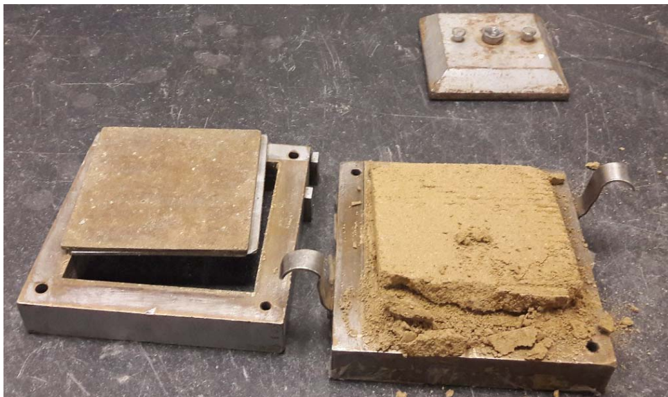
Fig. 3: Soil sample after testing (Direct shear).
