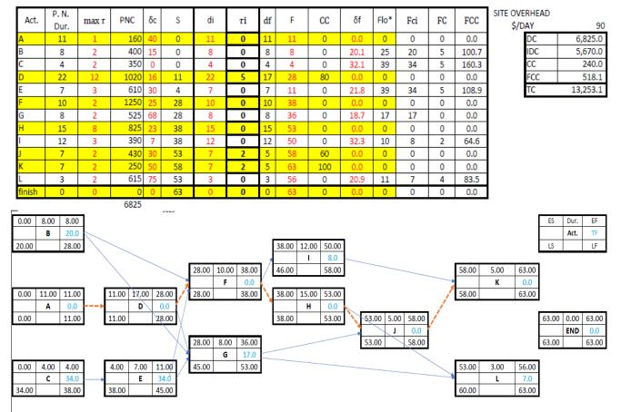
Fig. 5. Probabilistic Crashed Network Diagram with Float Consumption
