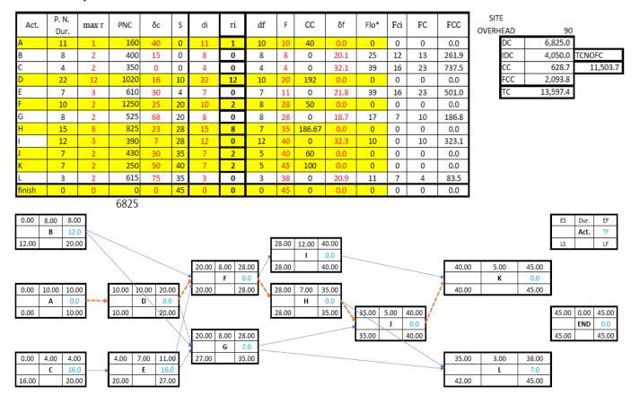
Fig. 6. Probabilistic Crashed Network Diagram without Float Consumption
