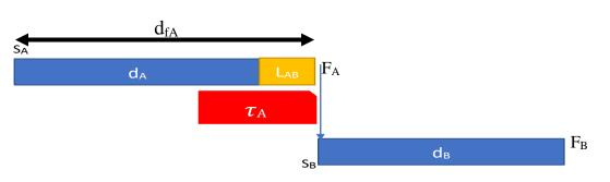
Fig. 4. The Precedence Constraint for the FS Relationship
