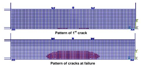
Fig. 10 Patterns of 1st crack and the cracks at failure for control RC beam
