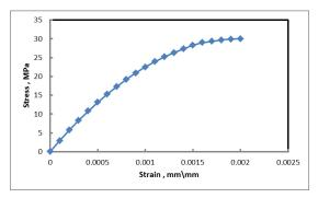
Fig. 3 Stress - Strain Curve for concrete
