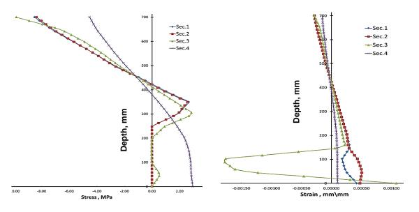
Fig. 9 Distribution of normal stress and normal strain for the selected sections in control RC beam
