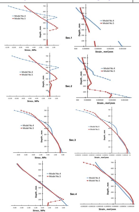
Fig. 15 Distribution of normal stress and normal strain for the selected sections in drilled RC beam
