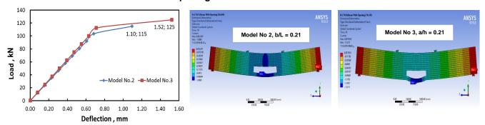
Fig. 11 Load - deflection of RC beams with opening and their patterns in numerical analysis
