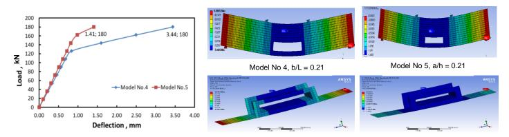
Fig. 14 Load deflections of RC beams with opening and CFRP and their patterns through numerical analysis
