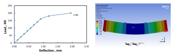
Fig. 7 Load - deflection of control RC beam and its pattern in numerical analysis
