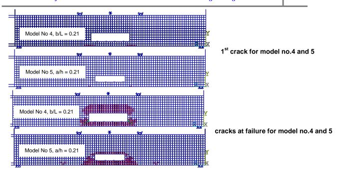
Fig. 16 Patterns of 1st crack and cracks at failure for RC beam model no.4 and 5
