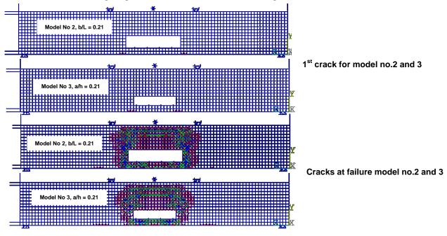
Fig. 13 Patterns of 1st crack and the cracks at failure for drilled RC beam, model No.2 and 3
