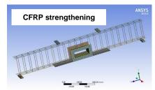
Fig. 6 Generated mesh for control RC beam, RC beam with opening and CFRP strengthening
