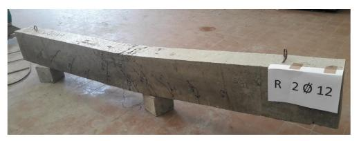
Fig.16: Failure mode of specimen (R 2Ø12), the first mode.
