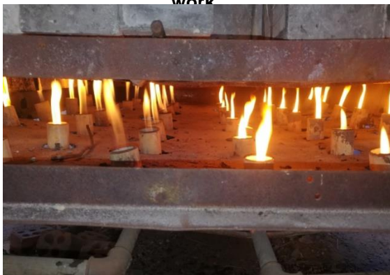
Fig. 3: Burning of Concrete specimens
