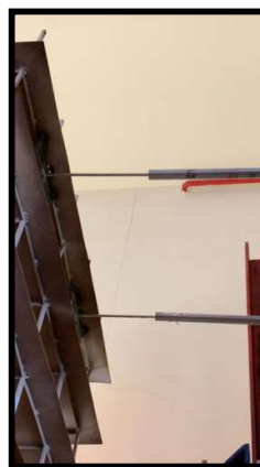
LVDTs at the top
