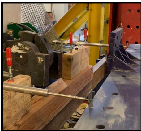
LVDTs at the bottom
