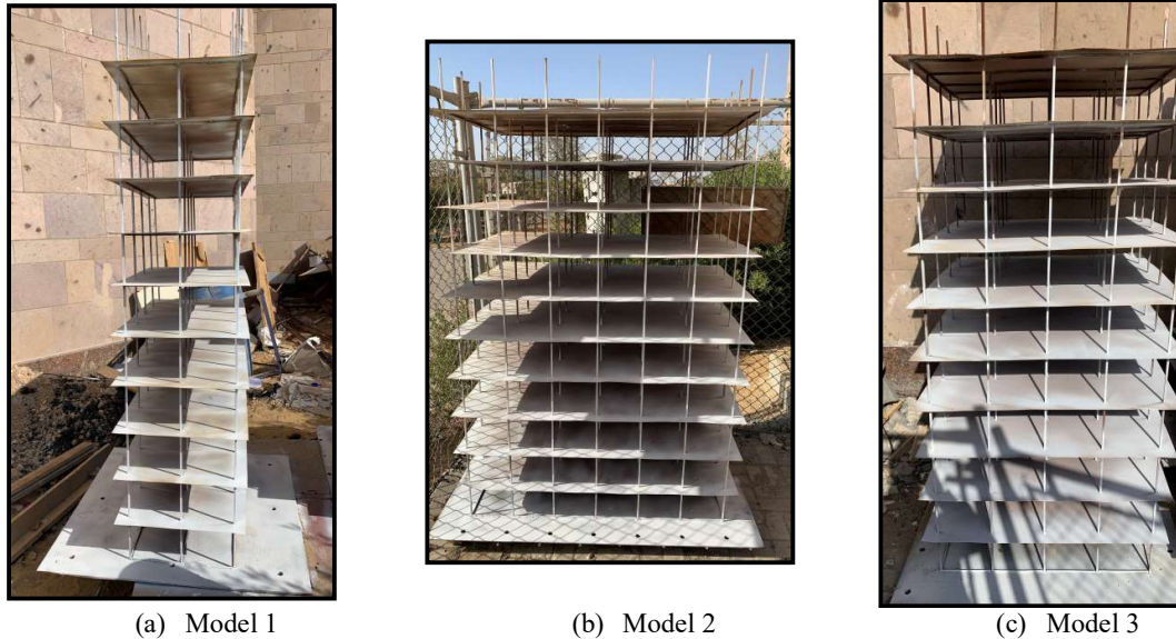
Figure 1. Fabricated steel structure models
