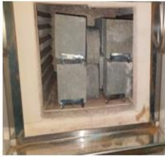
Fig3 Specimens inside the furnace
