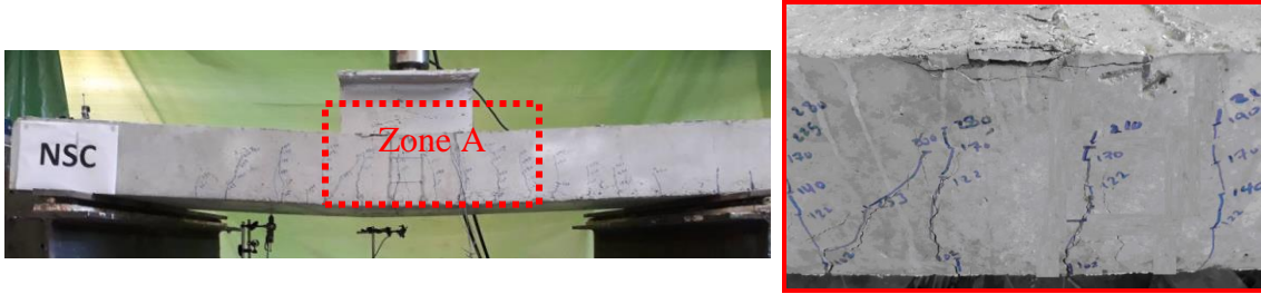
Fig. 5 Final crack pattern of specimen SN_{0.68\%,0} .
