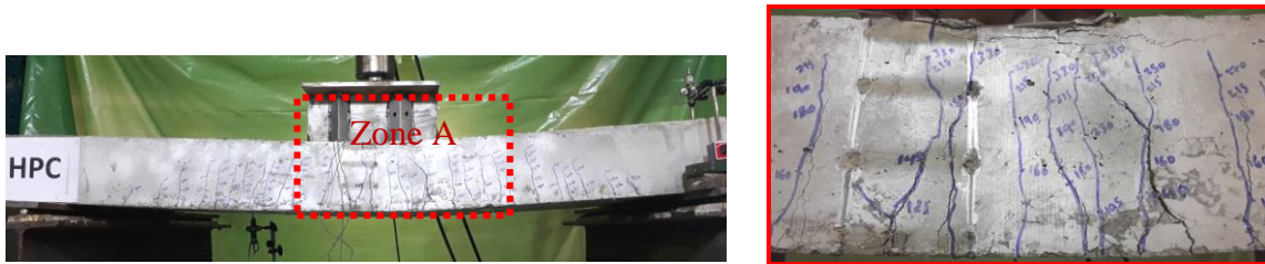
Fig. 6 Final crack pattern of specimen SH_{0.68\%,0} .
