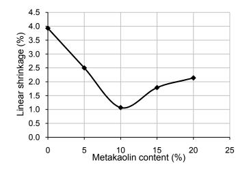
Fig. 3. Variation of shrinkage limit with metakaolin content
