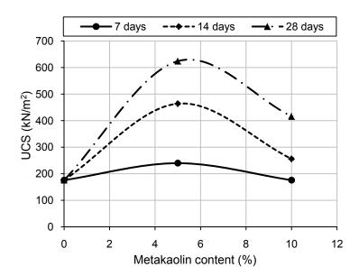
Fig. 6. Variation of UCS of clay soil - metakaolin
