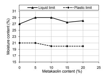
Fig. 2. Variation of atterberg limits with metakaolin content
