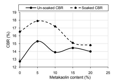
Fig. 5. Variation of CBR of clay soil - metakaolin
