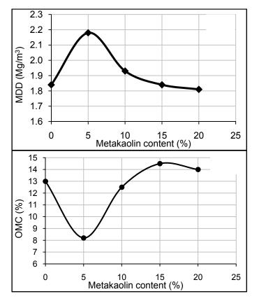
Fig. 4. Variation of (a) maximum dry density and (b) optimum moisture content of clay soil – metakaolin mixture
