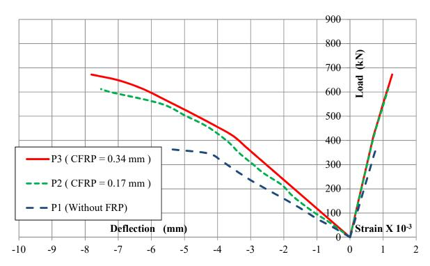
Figure (2) Effect of FRP Sheets Thickness on the Load-Deflection and the Load-Steel Strain Curves for Deep Beams P1, P2 and P3
