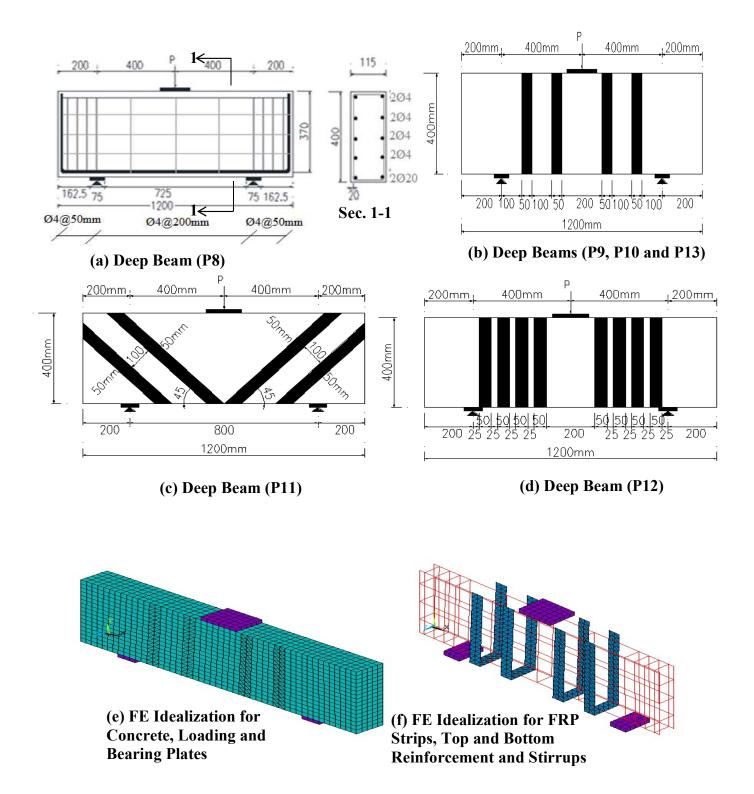
Figure (6) Typical Geometrical Details and F.E. Models for Deep Beams P8, P9, P10, P11, P12 and P13
