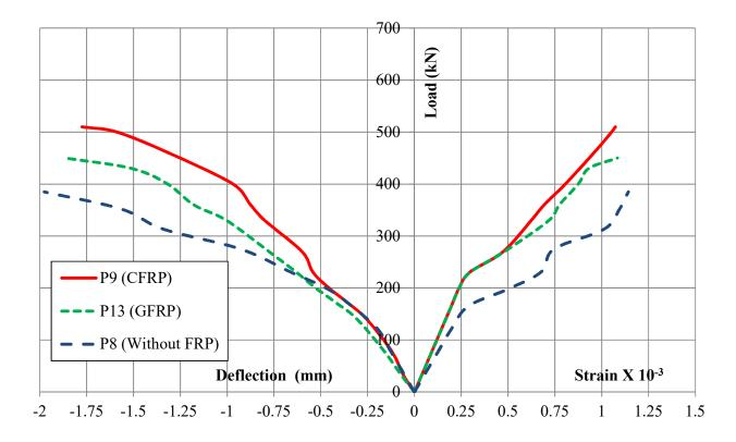
Figure (10) Effect of FRP Strips Material on the Load-Deflection and the Load-Steel Strain Curves for Deep Beams P8, P9 and P13
