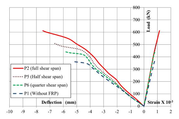
Figure (4) Effect of FRP Strengthening Length on the Load-Deflection and the Load-Steel Strain Curves for Deep Beams P1, P2, P5 and P6
