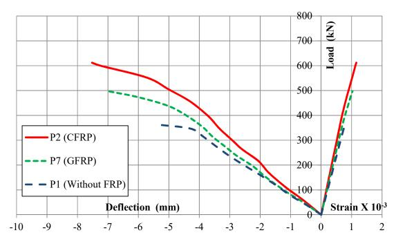
Figure (5) Effect of FRP Sheets Material on the Load-Deflection and the Load-Steel Strain Curves for Deep Beams P1, P2 and P7
