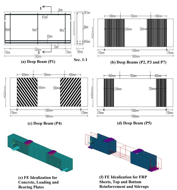
Figure (1) Typical Geometrical Details and F.E. Models for Deep Beams P1, P2, P3, P4, P5 and P7
