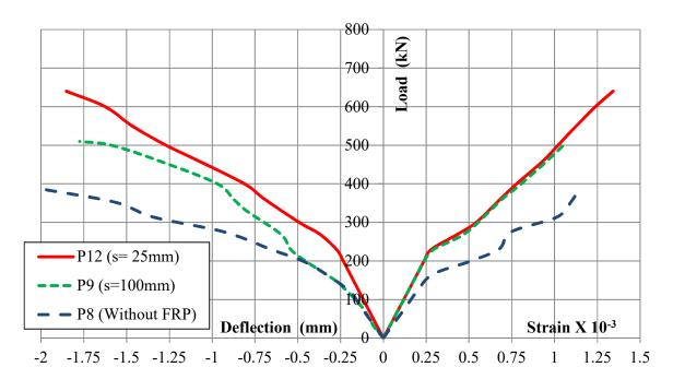
Figure (9) Effect of FRP Strips Spacing (S) on the Load-Deflection and the Load-Steel Strain Curves for Deep Beams P8, P9 and P12
