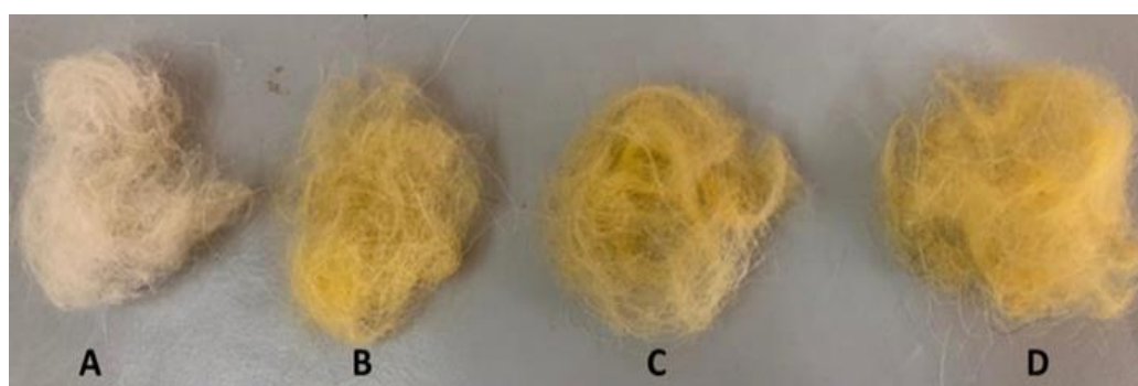
Fig. 1: Effect of different concentrations of the dyeing solutions Control (A), 1 mg/ml (B), 2 mg/ml (C), 4 mg/ml (D)
