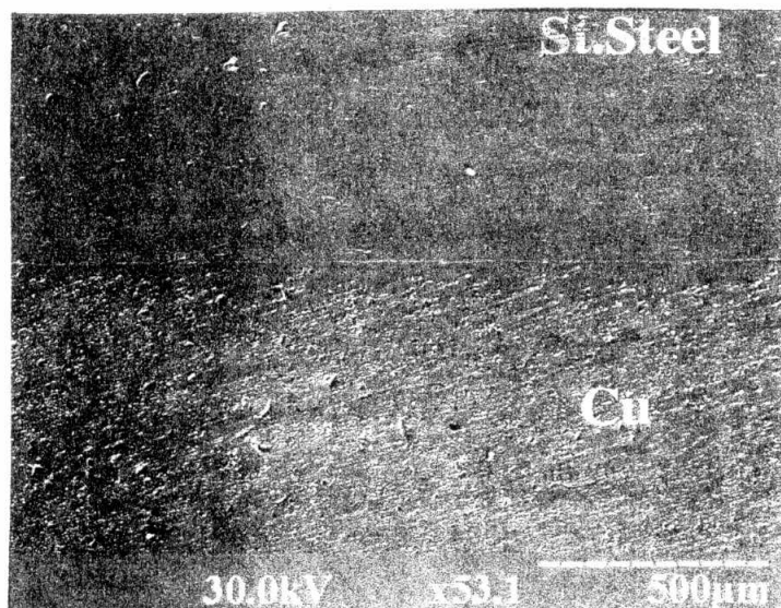
Fig. 8. Explosive welded joint of Stainless Steel and Copper-Nickel alloy obtained using a stand-off distance S=2 mm and an explosive ratio R=1.4.
