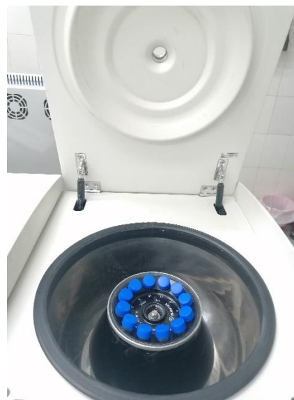
Figure (6): After 3 days solution centrifuge at 14,000 rpm for 5 min.
