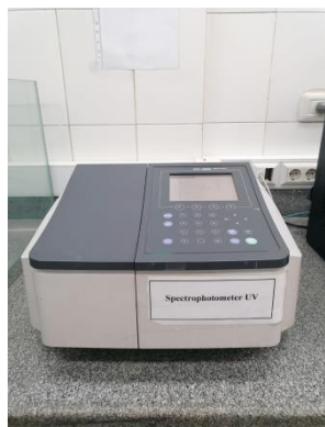
Figure (7): Shimadzu UV-1800 UV/Visible Scanning Spectrophotometer; 115 VAC, Japan.
