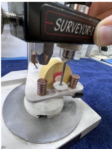
Figure (1): Surveyor modified device for standardization of discs polishing.
