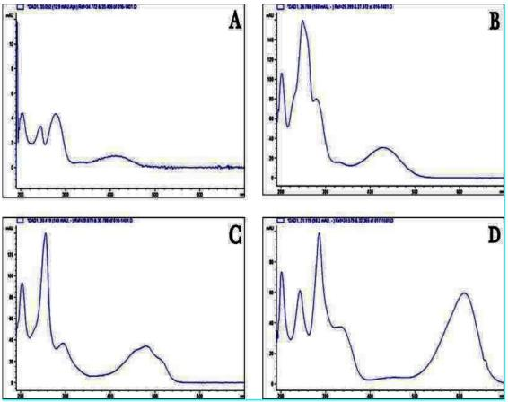
Fig. 4: UV-Vis absorption spectra for (A) Munjistin ,( B) Alizarin,( C )Puruprin ,( D ) Indigotin
