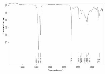
Fig.14. FTIR spectrum of F.oxysporum biodiesel.
