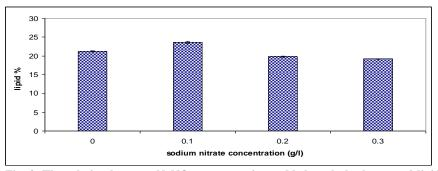
Fig. 3. The relation between NaNO<sub>3</sub> concentrations added to el-ghasheem and lipid percentage data plotted are means±SD of three replicates per test.
