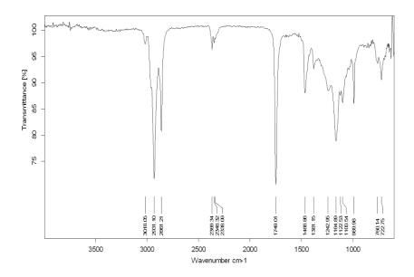
Fig.12. FTIR spectrum of lipid extracted from *F.oxysporum* using 125 gl<sup>-1</sup> elghasheem plus 0.1 gl<sup>-1</sup> NaNO<sub>3</sub> medium .
