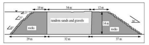
Fig.1. Note. Cross section of the structure of the Sadd el Kafara dam. From Sadd-el-Kafara: the world's oldest large dam. International Waterpower & Dam Construction by G. Garbrecht, 1985, International *Water Power & Dam Construction*, *37*, p. 74.
