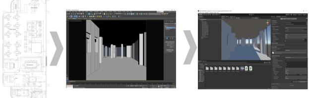
Figure 6: the preparation of simulation model from 3dmax to Unity author
