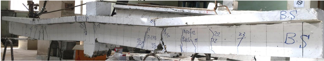
Fig. 4. Failure mode of beam BS1.
