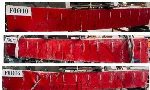
Fig. 9: Crack pattern of specimens in Group 3 at failure
