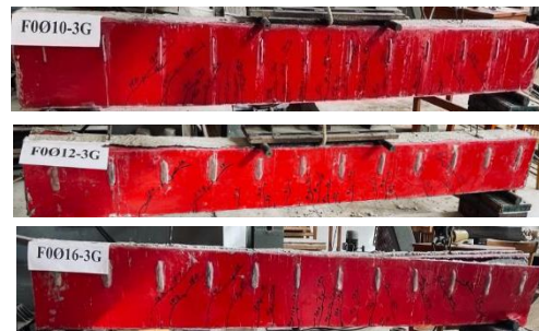
Fig. 10: Crack pattern of specimens in Group 4 at failure
