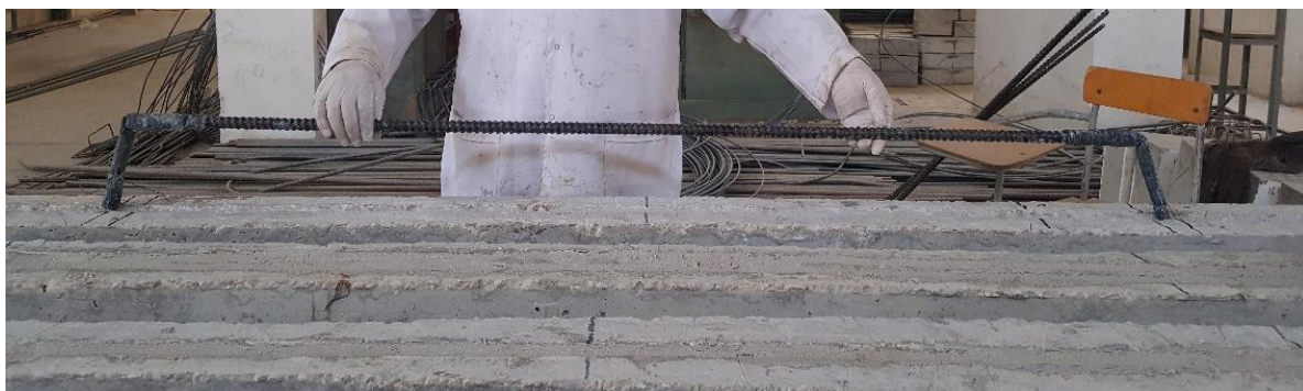
Fig. 4: Installation of the anchored BFRP bar
