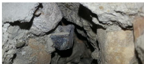
Fig. 12: Fatigue failure due to a rupture in the reinforcing steel bar
