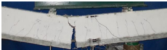
Fig. 10: failure mode of BU
