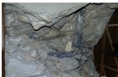
Fig. 12: Fatigue failure due to a rupture in the reinforcing steel bar
