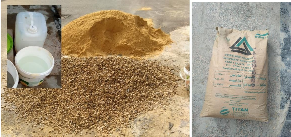
(a) Preparing the components; water, sand, dolomite and Portland Cement sulphate resistant
