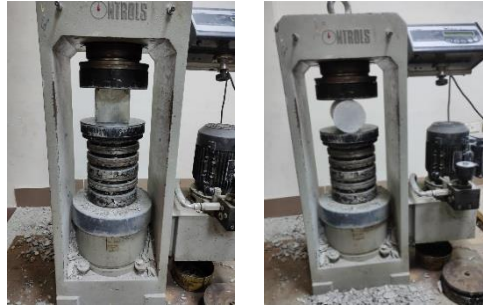
(a) Compression test of cubes (b) Splitting test of cylinders
