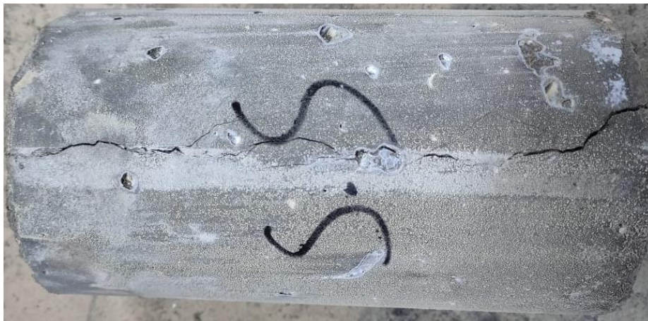
Fig. 6 Failure pattern of cylindrical sample of S-S group after splitting tensile test at curing age 28 days.
