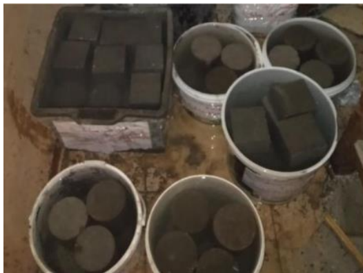
(e) Curing by immerge in isolated tanks
